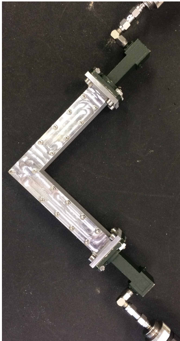
(a) Photo of the waveguide bend connected to a VNA.
