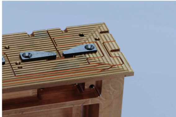
(d) Bottom half of the array block. Here, the soft iron pole pieces are shown placed in their pockets. Normally they are attached to the upper half of the block.
