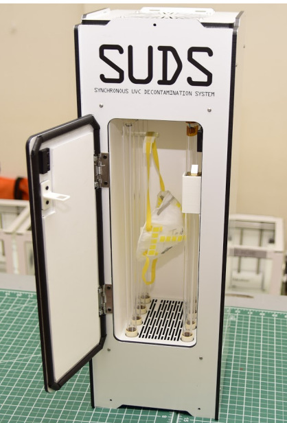
Case Western's SUDS (Synchronous UV Decontamination System), An open source UV mask decontamination solution for nurse stations, is now being brought to market by a medical device firm. Source: Case Western University / Sears think[box]
