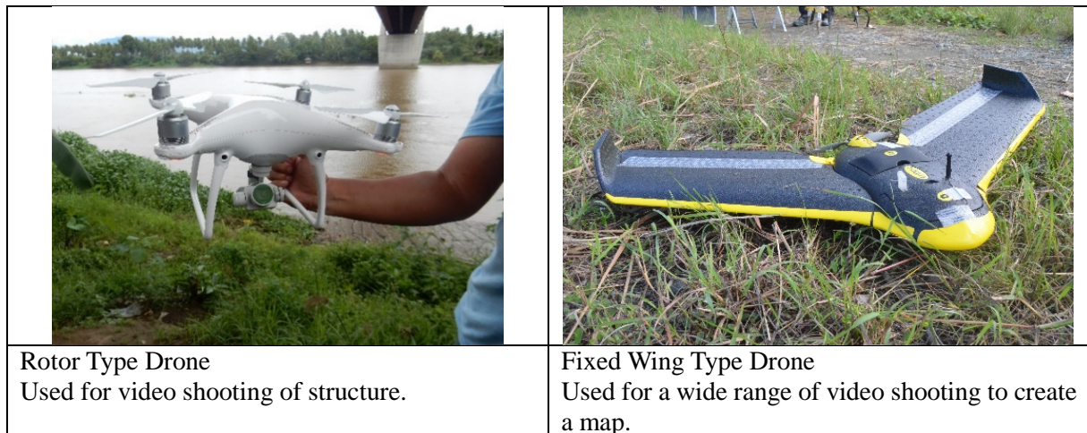
Figure 1.3.3.3-1 Drones used for Inspection
