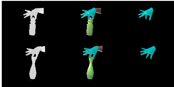
Figure 2. The hand tracker used in the in-hand scanning pipeline. The left image shows the raw depth input map, the middle image shows the hand pose overlaid on top of the RGB-D data, while the right image shows just the hand pose.
