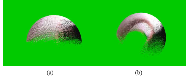
Figure 4. Reconstruction without (a) and with (b) hand motion capture on synthetic data generated from [1]. Since the visual correspondences alone are not descriptive enough for symmetric objects, the reconstruction collapses to a hemisphere (a). On the contrary, the use of hand motion capture gives meaningful contact correspondences , successfully driving the reconstruction process (b). The clear observation of the occlusions by the manipulating fingers (b) indicates a sensible registration. The motion includes some notable translation and rotation, but the object is not fully rotated in order to allow for a complete reconstruction.
