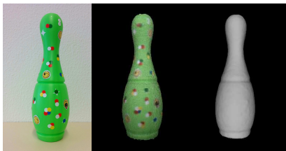
Figure 7. The bowling-pin object enriched with 2d texture using stickers (left). The added texture allows for the reconstruction of a reference ground truth shape (middle, right) facilitating quantitative evaluation.
