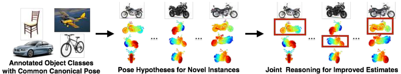
Figure 2. Overview of our approach. We first induce pose hypotheses for novel object instances using a system trained over aligned annotated classes (Section 2). We then reason jointly over all instances of the novel object class to improve our pose predictions (Section 3).
