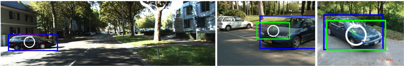
Figure 14: Examples of wrong detections or pose estimations. These cases include: missed detections due to wrongly adjusted bounding box caused by bad viewpoint estimation; missed detections of objects outside image boundary; and bad viewpoint caused by opposite view similarity.
