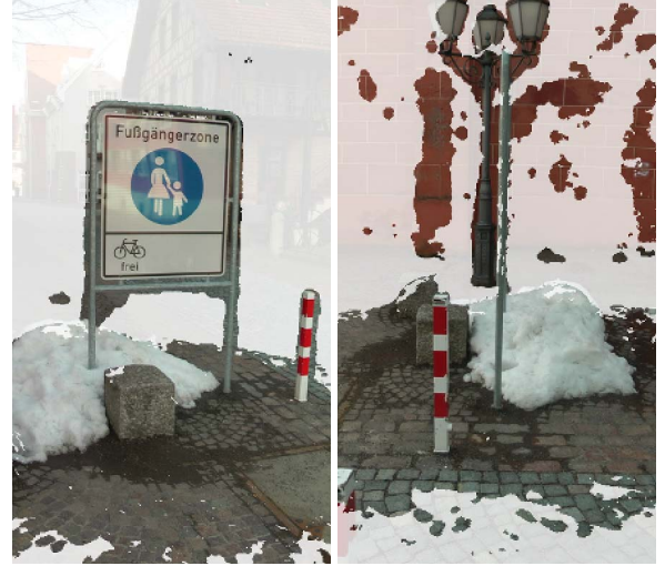
Figure 6. Two of the 50 input images of the street sign scene. The highlighted pixels contribute to the reconstruction and are represented in the point cloud. The total number of points is about 5 million.
