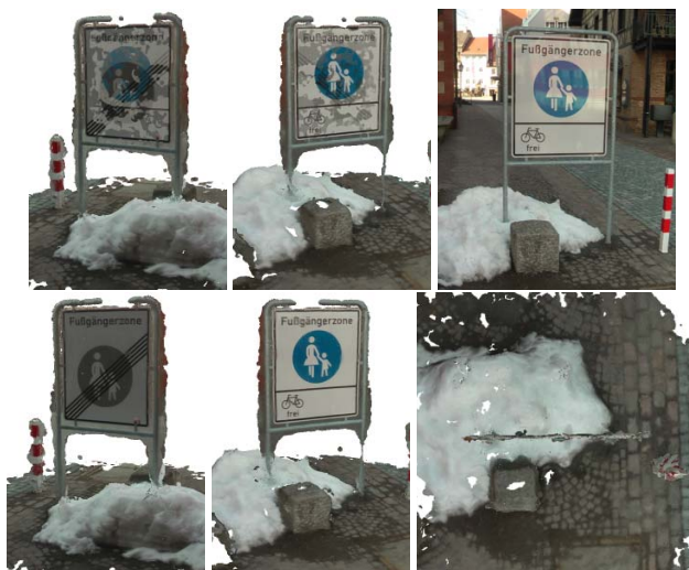
Figure 1. Dense point cloud reconstruction of a street sign. Top: Two renderings of the reconstruction when ignoring opposed surfaces (left and center) and a photo of the scene (right). Many points are on the wrong side of the object. Bottom: Reconstruction result of our approach explicitly modeling opposed surfaces. All images are rendered with front- and back-faces visible. Our approach resolves collisions between points that represent different sides of thin objects. Almost all points from the correct side pass the depth test (left and center) and therefore lie on the correct side. The approach preserves the thin structure of the objects, as seen in the view from the top (right).
