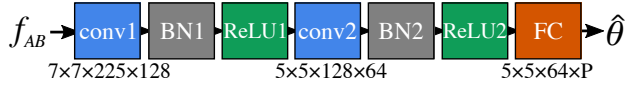
Figure 4: Architecture of the regression network. It is composed of two convolutional layers without padding and stride equal to 1, followed by batch normalization and ReLU, and a final fully connected layer which regresses to the P transformation parameters.
