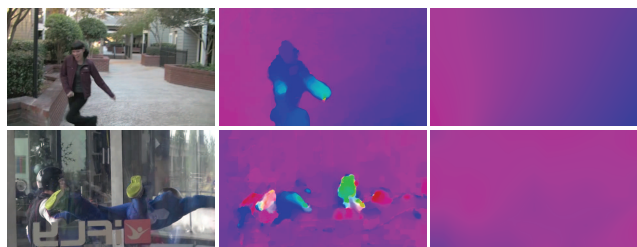
Figure 9: Foreground motion removal. Left : input images. Middle : Conventional optical flow. Right : Our flow from the warped mesh.
