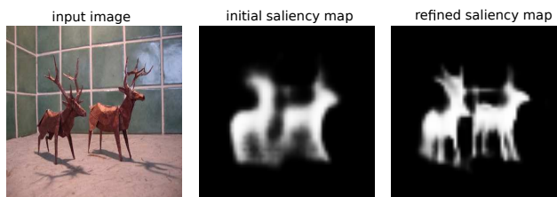
Figure 1. An example of applying recurrent attention-based saliency refinement to an initial saliency map produced by convolutional-deconvolutional network. Compared to the initial saliency map, the refined saliency map has significantly sharper edges and preserves more object details.
