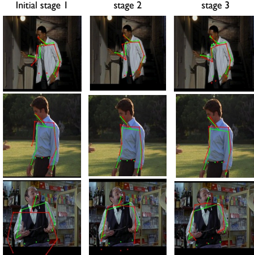
Figure 6. Predicted poses in red and ground truth poses in green for the first three stages of a cascade for three examples.
