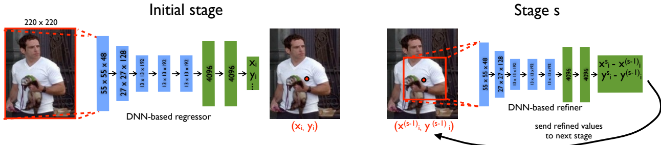
Figure 2. Left: schematic view of the DNN-based pose regression. We visualize the network layers with their corresponding dimensions, where convolutional layers are in blue, while fully connected ones are in green. We do not show the parameter free layers. Right: at stage s , a refining regressor is applied on a sub image to refine a prediction from the previous stage.
