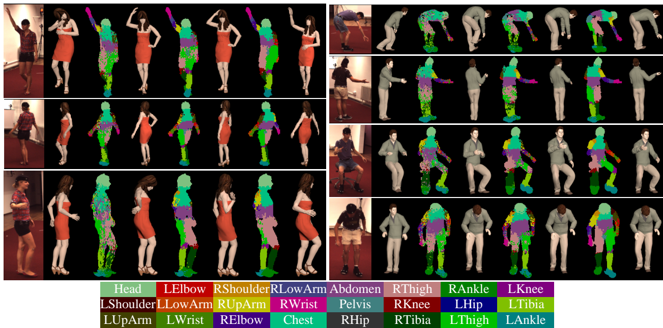
Figure 4: Examples of labeling inference and 3D human pose estimation for our different models. The columns represent from left to right: the input image, the 3D pose predicted by a HoG baseline, then labeling and estimated 3D pose for our RF, rIRF and rlpRF models.
