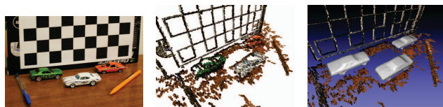
Figure 10. Reconstruction of multi-object scenes. (Left) 1 out of 10 input images. (Middle) MVS [14]. (Right) Our reconstruction.
