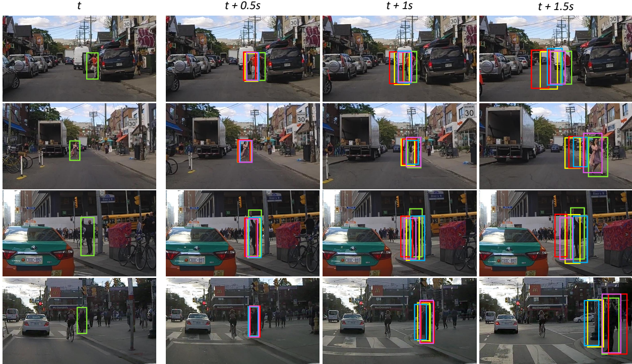
Figure 5. Examples of trajectory prediction algorithm using the proposed model PIE_{traj} with different input combinations. The color and model combinations are: loc (yellow), loc+PIE_{int} (blue), loc+PIE_{speed} (red), and loc+PIE_{int}+PIE_{speed} (purple). Ground truth annotations are shown in green. The sequences depict different traffic scenarios. From top to bottom: A man leaving his vehicle, a woman crossing the street, a man hailing a taxi, and a woman waiting to cross.
