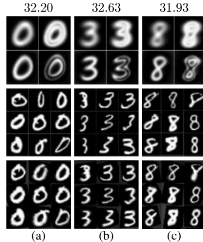
Figure 8. Congealing results of the proposed method on 1 000 000 images per digit from infiMNIST. (a)-(c) correspond to different digits. Top: mean (first columns) and variance (second columns) images, before (first rows) and after (second rows) alignment. Middle: a subset of the actual inputs. Bottom: a subset of the actual outputs. APSNR for each digit is reported at the top of each subfigure.
