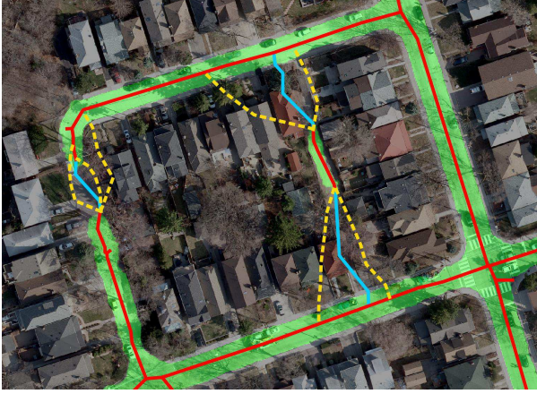
Figure 3: Segmentation softmax is highlighted in green, the extracted road center line is shown in red, and the connection hypotheses generated by the A^* search are in blue. Dashed yellow shows other possible connections which were not selected by the A^* algorithm.
