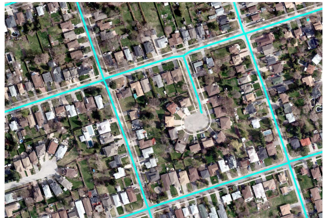
Figure 1: Road topology from aerial images at a large scale. Our extracted road network is shown in blue.
