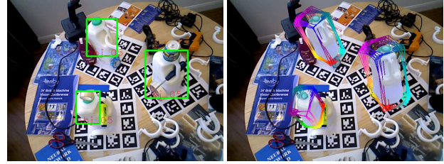
Figure 9: One failure case where incorrect bounding box regression, induced by occlusion, led to wrong 6D hypothesis creation. In such cases a subsequent refinement cannot always recover the correct pose anymore.
