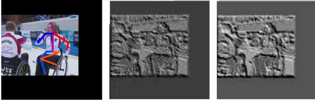
Figure 3: Examples of features before and after an 1 \times 1 convolutional layer. Often the features are copied over with little modifications, usually consisting in the details’ removal. The contrast was altered for better visualization.
