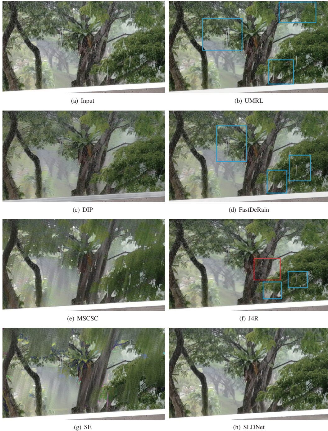
Figure 3. Visual comparison of different deraining methods on a real rain video sequence. The remaining rain streaks and artifacts are denoted with blue and red boxes, respectively. Note that, two white vertical lines in the center of the figure are parts of tree textures instead of rain streaks.
