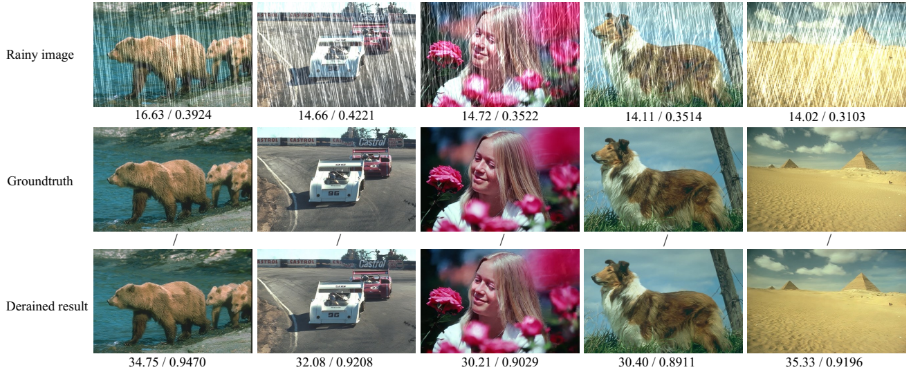
Figure 11. (a) The first row: 5 representative rainy images with different rain densities and directions involved in Rain100H. (b) The second row: the corresponding groundtruth. (c) The third row: The derained results of our RCDNet. PSNR/SSIM are listed below the corresponding images for easy reference.
