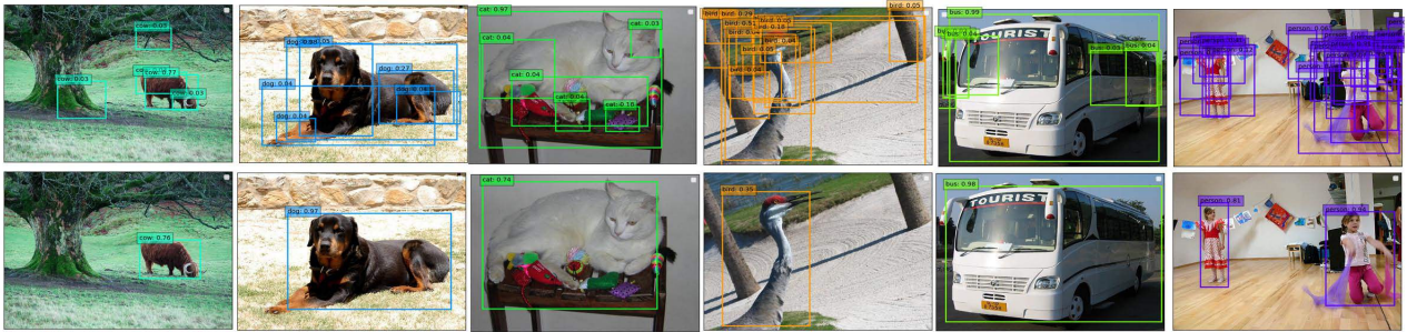
Figure 5. Qualitative results on PASCAL VOC. Images in the top row shows the object predicted by Xnor-Net, while the images with the objects detected by our BiDet are displayed in the bottom row. The proposed BiDet removes the information redundancy to fully utilize the network capacity, and learns the sparse object priors to eliminate false positives (best viewed in color).
