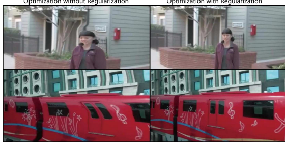
Figure 3. Video stabilization results using regularization vs. no regularization. (Left) Due to the moving object in the scene and the inaccurate original optical flow, unexpected artifacts are introduced if the video is stabilized purely according to optical flow. (Right) Applying proper regularization helps reduce the visual artifacts.
