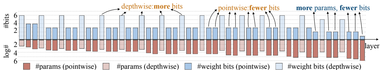
Figure 5: Quantization policy under model size constraints for MobileNet-V2. Our RL agent allocates more bits to the depthwise convolutions, since depthwise convolutions have fewer number of parameters.
