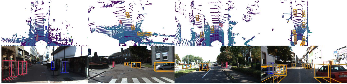
Figure 3. Qualitative analysis on KITTI. We show a bird’s eye view of the lidar point cloud (top), as well as the 3D bounding boxes projected into the image for clearer visualization. Note that our method only uses lidar. We show ground truth (gray) and predicted boxes for car (orange), cyclist (red) and pedestrian (blue). The box orientation is shown by a line from the bottom center to the front of the box.
