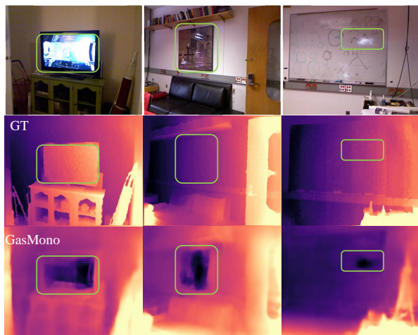
Figure 7. Limitations of GasMono. Since GasMono is trained in a self-supervised manner, it cannot estimate a reasonable depth for those regions with photometric changes.
