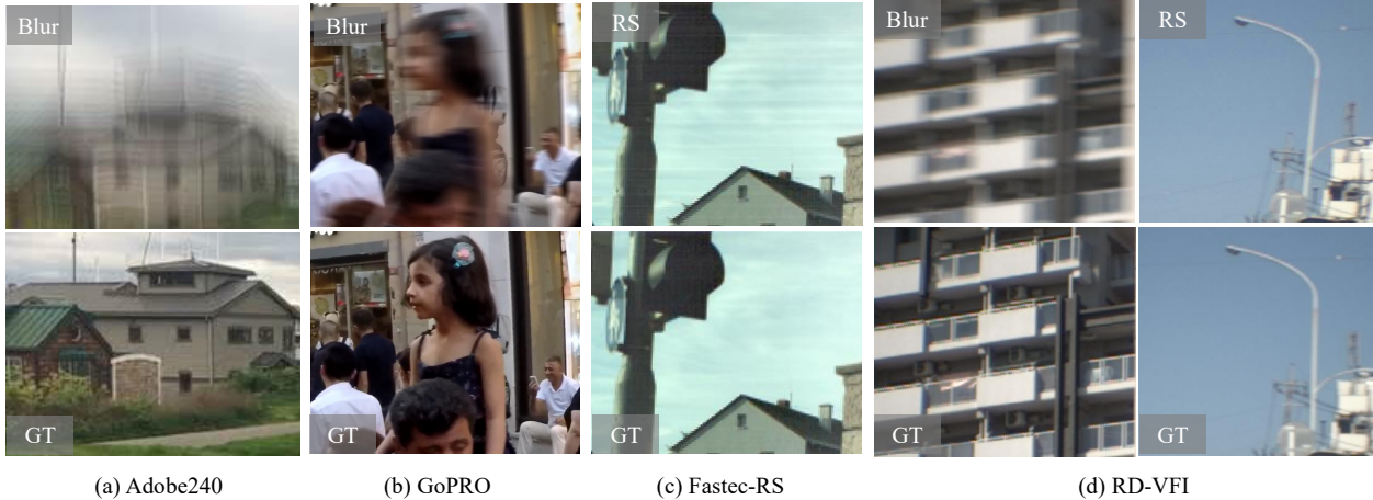
Figure 1: Samples from the existing synthetic dataset and our RD-VFI dataset. (a) and (b) are samples from Adobe240fps and GoPRO, respectively. The unnatural hops and steps caused by the discontinuity of averaging process can be easily spotted. (c) are samples from Fastec-RS with horizontal streak artifacts. (d) are from our real-world dataset RD-VFI.
