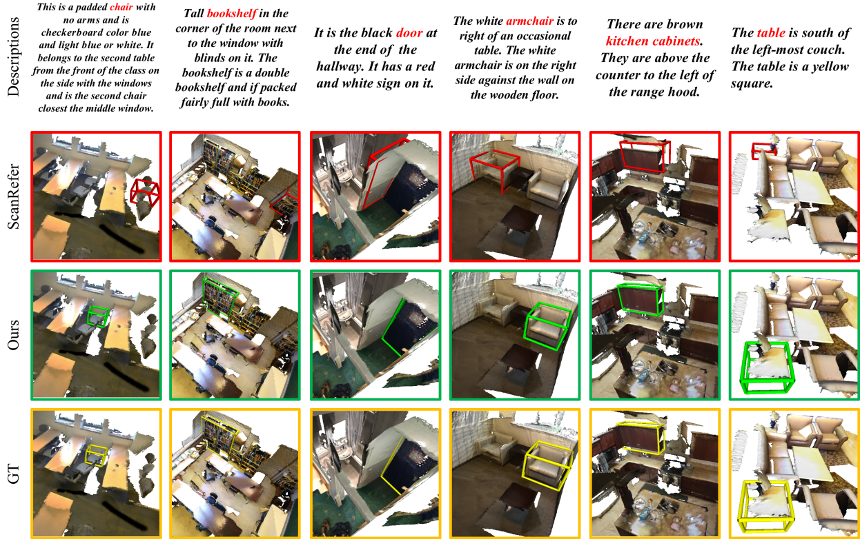
Figure 5. Qualitative results from ScanRefer and our InstanceRefer. Predicted boxes are marked green if they have an IoU score higher than 0.5, otherwise they are marked red. The ground truth boxes are displayed in yellow.
