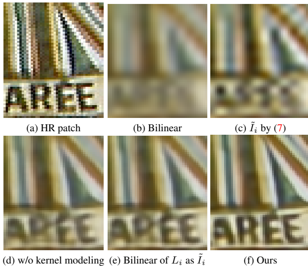
Figure 7. Effectiveness of the blur kernel estimation on video SR ( \times 4 ). Using blur kernel estimation is able to generate the results with clearer structural details.
