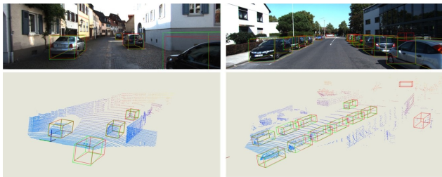
Figure 7: Qualitative 3d detection results on KITTI validation set. Red boxes represent our predictions, and green boxes come from ground truth. LiDAR signals are only used for visualization.
