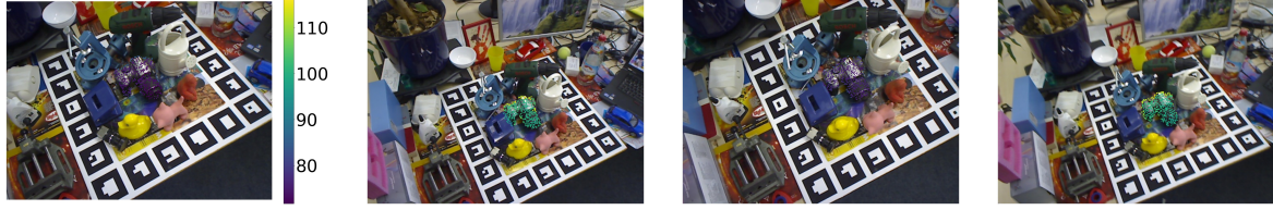
(a) 3D point clouds \mathbf{X}_1, \mathbf{X}_2, \mathbf{X}_3, \mathbf{X}_4 are projected onto corresponding frames. Colorbar shows depth in cm.
