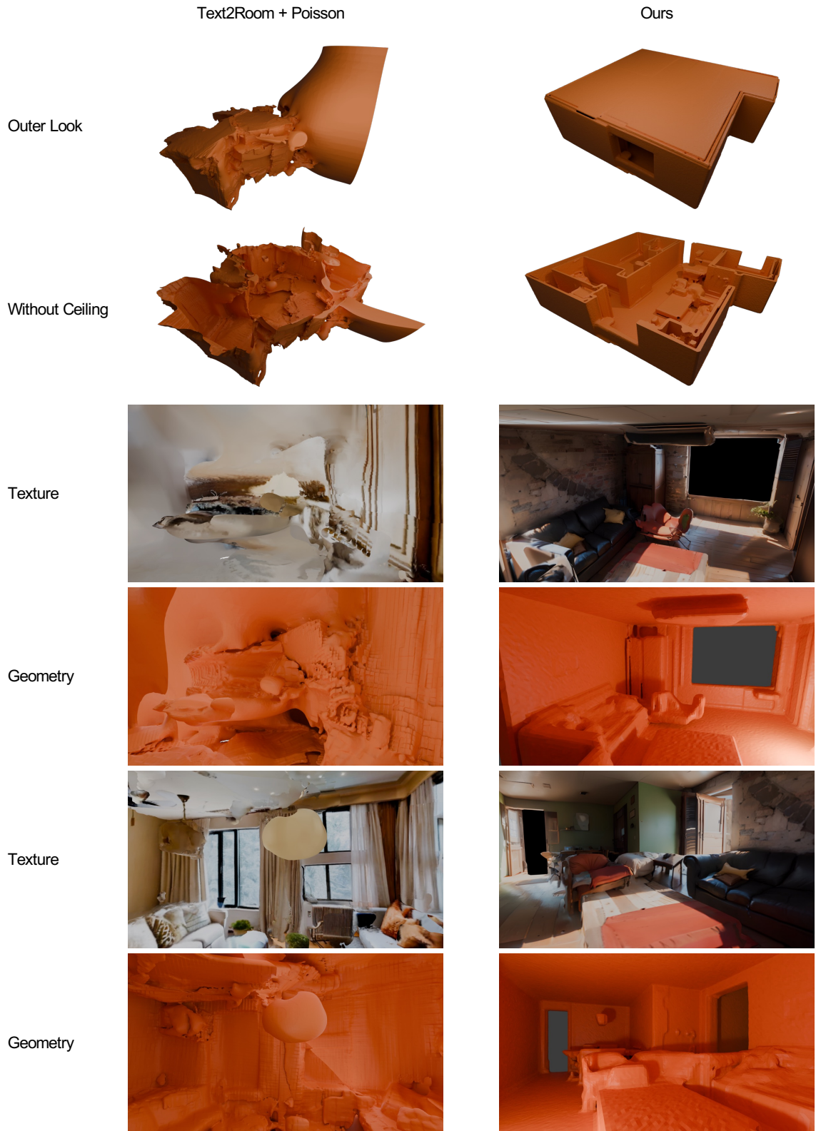
Figure 12. Comparison of Text2Room and our approach in larger views. As previous Fig. 5 shows, Poisson reconstruction significantly improves the performance of pure TextRoom, so that here we only demonstrate the results of Text2Room [5] + Poisson [8]. The textures of our results are produced by DreamSpace [14] as a post-processing of scene geometry generation.
