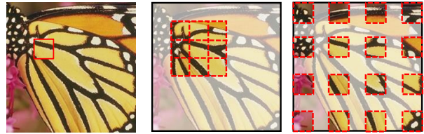
Figure 4. An illustration of sampling strategies. The original image with the highlighted image node (left), local sampling (middle), and global sampling (right) are demonstrated. In this way, image graphs could flexibly gather both local and global information in an efficient manner.
