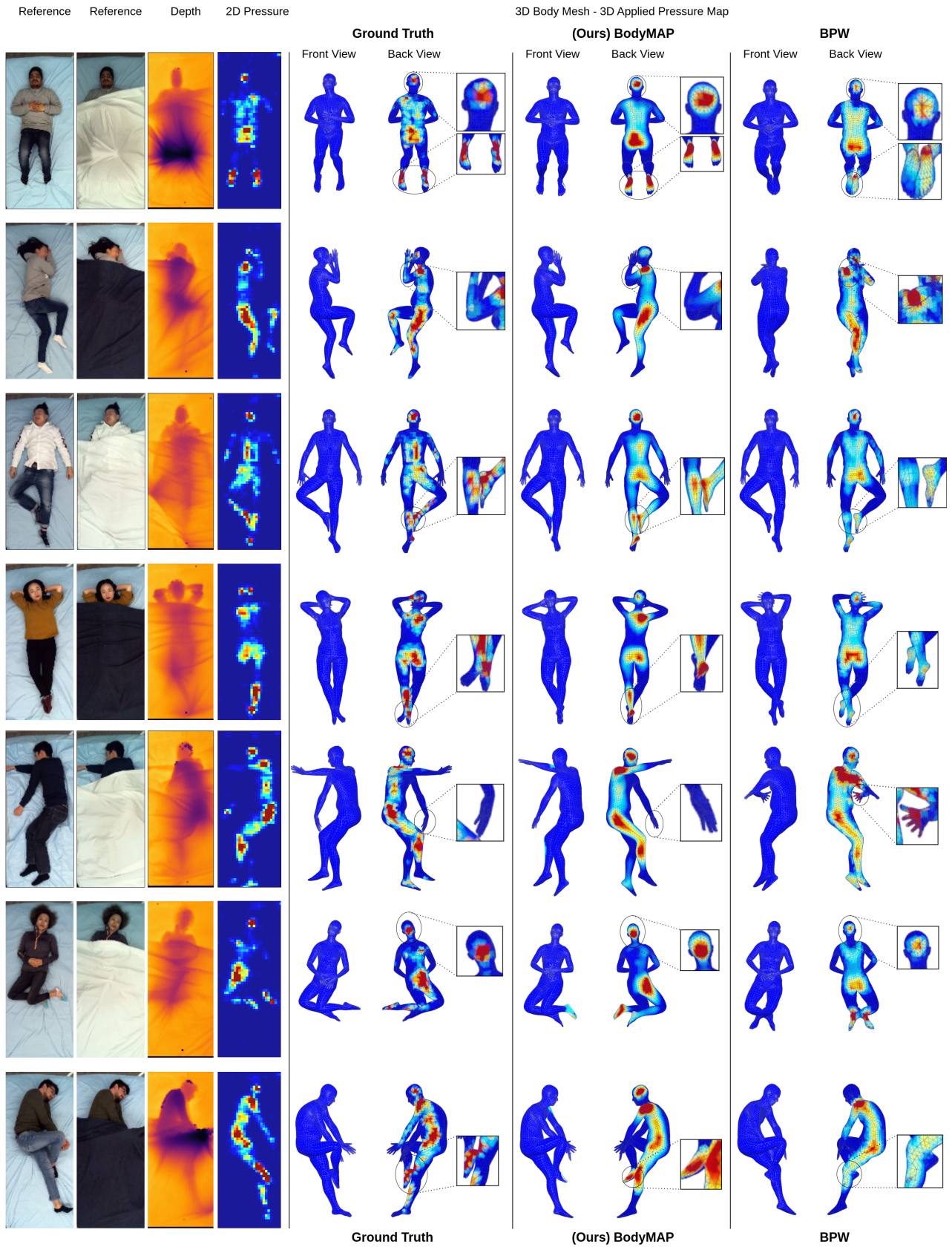
Figure 4. Results of inferring body mesh and 3D applied pressure map for examples from the SLP [25, 27] test set.
