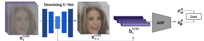
Figure 4. Distribution guidance in the h-space . For a given batch \mathbf{x}_t^{[1:N]} , we extract the intermediate h-space representation \mathbf{h}_t^{[1:N]} and pass it through ADP to obtain attribute distribution \hat{\mathbf{p}}_\theta^a . Guidance updates \mathbf{h}_t^{[1:N]} by backpropagating the derivative of loss.
