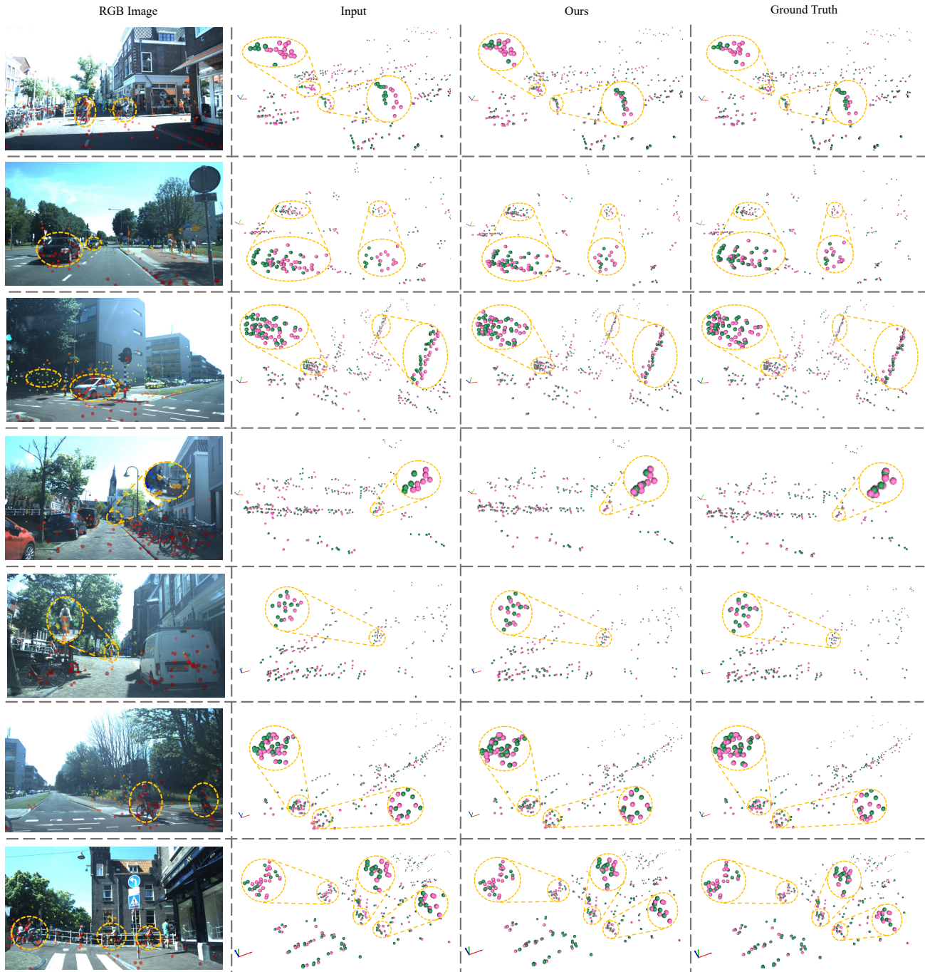
Figure E. Qualitative scene flow results in seven Test scenes. From left to right: 1) radar points from the source frame projected to the corresponding RGB image (points are coloured by distance from the sensor), 2) two input radar point clouds, the source one (pink) and the target one (green), 3) the source point cloud warped by our predicted scene flow and the target radar point cloud, 4) the source point cloud warped by ground truth scene flow and the target one. We mark regions of interest in amber and apply the zooming-in operation for them.
