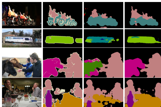
Figure 4. Qualitative results on Pascal VOC2012 using 183 fine labels. Columns from left to right denote the original images, the ground-truth, the supervised segmentation results, and the iMAS segmentation results, respectively.
