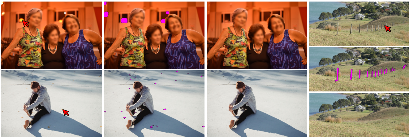
Figure 1. We present a pipeline that enables the automatic segmentation of distractors in photos using a single click. With just one click, our pipeline can detect and mask the distracting object in the photo and identify other similar objects that may also be causing distraction. We can then use popular photo editing tools such as Adobe Photoshop’s ‘Content-Aware Fill’ to remove the visual distractions seamlessly. Each triad shows the input images with a click, segmentation results, and photo editing performance.
