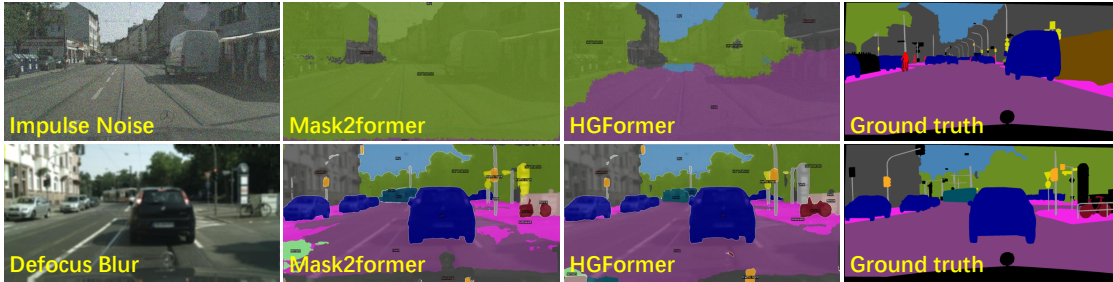
Figure 5. Visualization of results on corruptions. We choose two kinds of corruption at level 5 for this visualization: impulse noise and defocus blur. The models are trained on Cityscapes.
