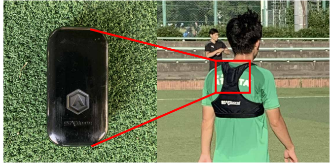
Figure 3. GNSS devices used in the measurement experiment. Athletes inserted the device inside a special vest to prevent the device from falling.
