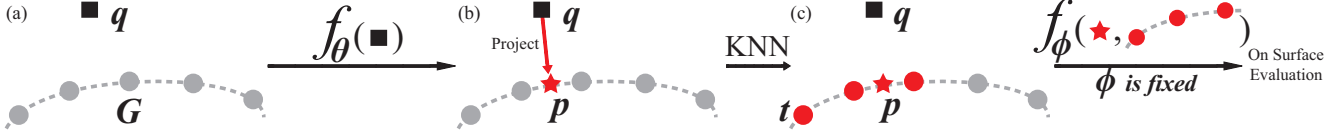
Figure 1. The demonstration of our method during test. We leverage a data-driven strategy to learn on-surface decision function f_\phi as an on-surface prior during training. During testing, we learn SDFs f_\theta from a sparse point cloud \mathcal{G} . (a) Query q is sampled around \mathcal{G} . (b) q is projected into a projection p towards \mathcal{G} using the path determined by SDFs f_\theta . f_\phi evaluates whether p is on the surface represented by the K nearest neighbors t of p in (c). We run the marching cubes to reconstruct surfaces of f_\theta .
