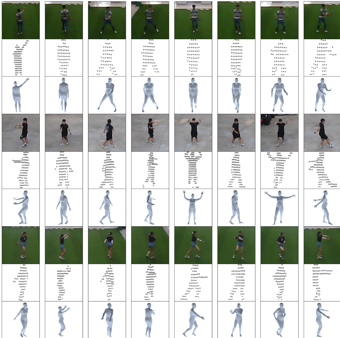
Figure 5. 3D capturing results on long-range human motions. For each body motion, the top row shows the reference images, the middle row shows the input LiDAR points, and the bottom row shows the captured motion results on the LiDAR view.
