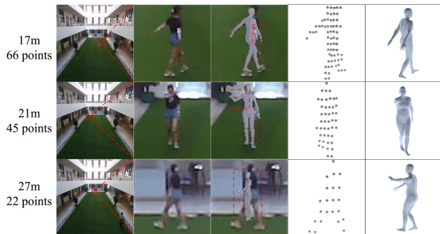
(b) The qualitative results over the chosen three distances. The columns from left to right are the original images, the enlarged images, VIBE results, the point clouds, and our results.
