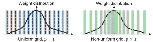
Figure 2. Example of the proposed parametric non-uniform grid in comparison with a uniform grid for  $n = 4$ .
