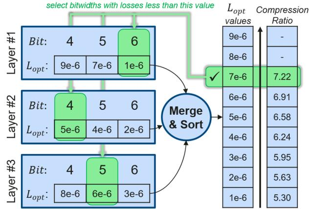
Figure 3. The scheme of the bitwidth selection procedure. Example for SCR equal to 7.
