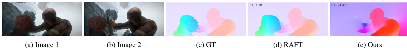
Figure 6: An example failure case. When the scene contains significant featureless regions or motion blur, top- k correlations may not contain the correct matches and can lead to incorrect flow prediction.
