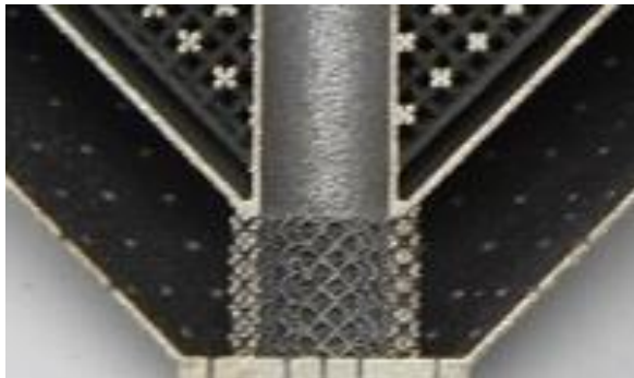
Flow distributor lattice structure (Octet-Truss 30%RD) to improve radial flow spatial distribution.
