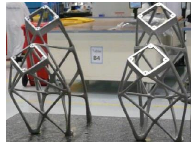
Topology Optimized AM Scalmalloy antenna struts currently on-orbit. Courtesy Begoc, 2019*.
