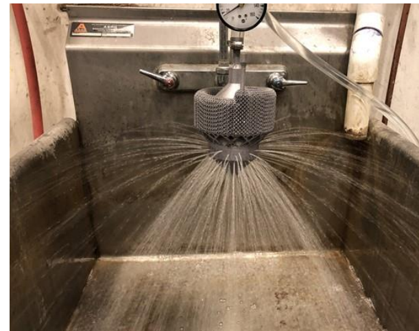
TVS Augmented Injector V4 (AlSi10Mg) water flow test and LN 2 tests.
