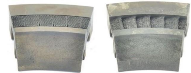
IN718 stator segments pre-etch (left) and post-etch (right). Supports dissolved sufficiently to remove via a grit blasting.
