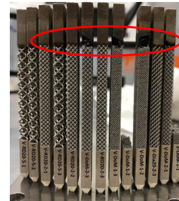
Discrete transition burn-out (IN718). Gradient transition optimized specimens (IN718).
