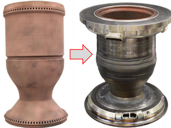
EB-DED Inco 625 Jacket on L-PBF GRCop-84 Liner
