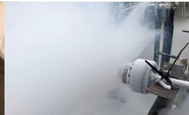
TVS Augmented Injector V4 (AlSi10Mg) water flow test and LN 2 tests.
