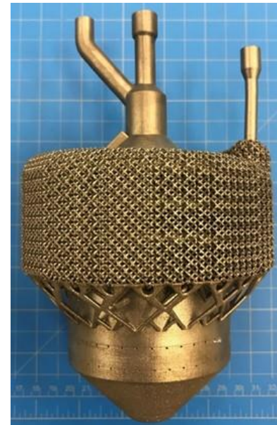
TVS Augmented Injector V4 (IN718), liquid circuit, 2-phase/gas circuit. Inner & outer lattice Dode-Medium (13 %RD)
