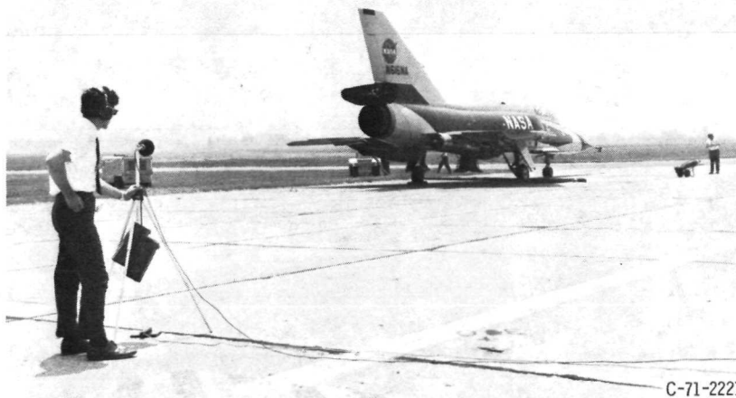
Figure 11. - Microphone position and orientation for static tests.
