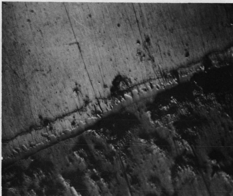
Fig. 2 - Typical intermetallic compound interface formed in specimens sheathed with bronze. Note irregular layer thickness. As Polished
