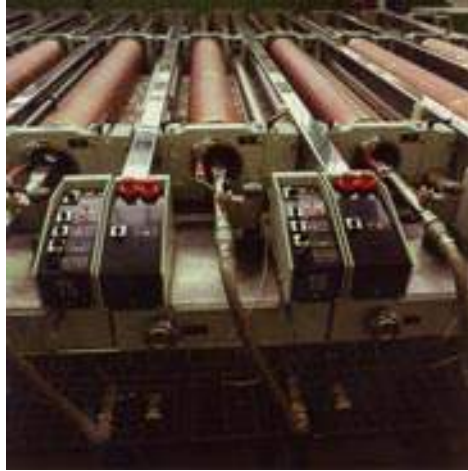
Figure 2.13 Rotary-screen printing machine showing printing heads, screens, connecting columns and screen drive shafts (Johannes Zimmer); one screen end-ring fits into a printing head (foreground) which includes squeegee support and setting fixtures; the end-ring at the far side is also driven by means of a drive shaft (left of screen); rectangular connecting columns on the left and right of the screen enable the position of the heads to be adjusted to suit various screen lengths
