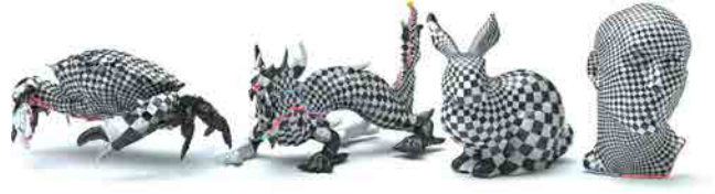
Fig. 14. The conformality of the embeddings: texturing the models using our embeddings shows they approximate conformal maps.
