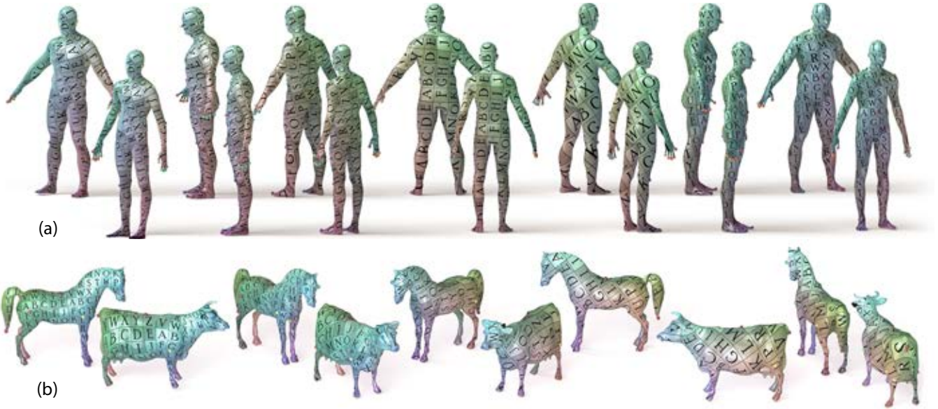
Figure 10: (a) A mapping between a pair of meshes from Figure 2, shown from seven different viewpoints; the map is guaranteed to be a homeomorphism between the two surfaces. Note that we re-texture the source mesh from each viewpoint. In (b) we show another mapping from several viewpoints.
