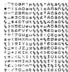
FIGURE 87: The VT220's glyphs from a ROM dump. VT100 implemented most of the first seven columns. Note the existence of box-drawing characters[75].
