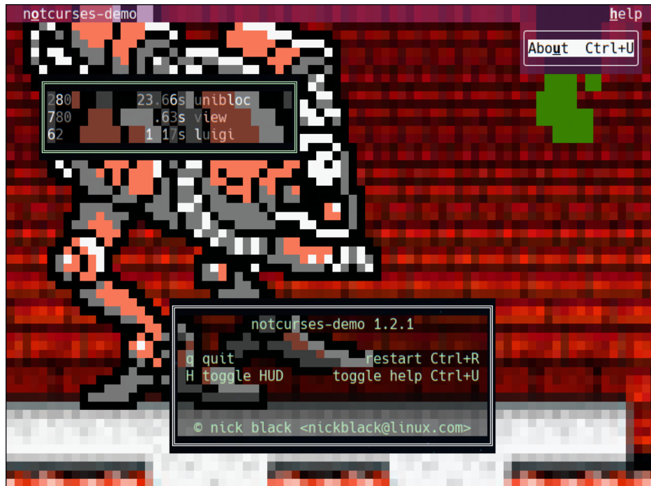
FIGURE 52: The notcurses-demo menu, unrolled in media res . Luigi, pursued by WarMECH, is leaping through the “Help” menu. In the upper left is the HUD, and at the bottom the About text, both implemented as translucent planes.
